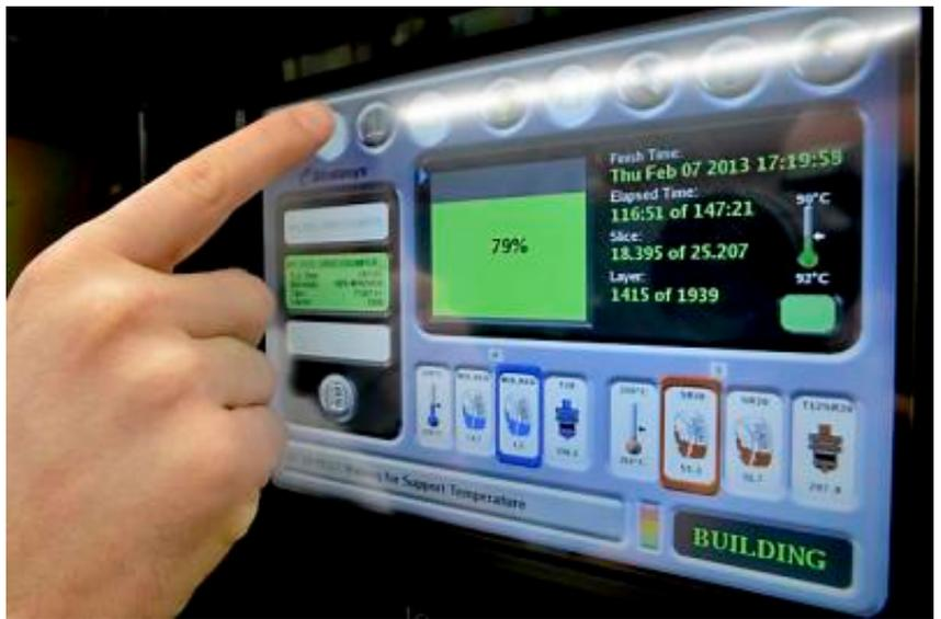
A control panel on the exterior of a "fused deposition modelling" printer is checked during the 3D "printing" of the thermoplastic front right bumper of a full-size car. (Pioneer Press: Richard Marshall)
