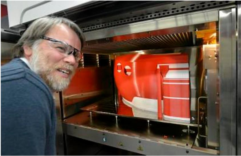
Jim Kor of Winnipeg, Manitoba, checks the progress of a car bumper, part of the Urbee 2 automobile, being printed with 3D technology at the RedEye facility of Stratasys in Eden Prairie on Wednesday February 6, 2013. (Pioneer Press: Richard Marshall)
