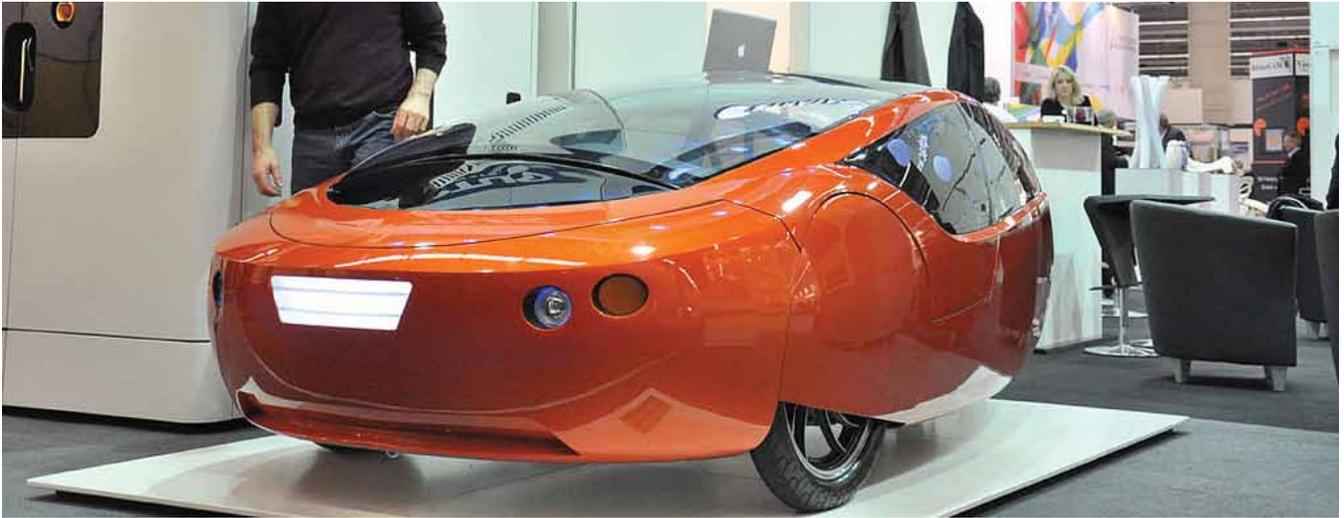
The Urbee's body is completely manufactured through Stratasys' 3D printing process, during which millimetre-thin layers of additive materials are stacked together to form complex objects.
